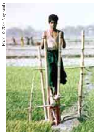
The Bamboo treadle pump designed by Gunnar Barnes and International Development Enterprises Nepal is manufactured in numerous small and medium-sized local workshops in Nepal and Bangladesh.
