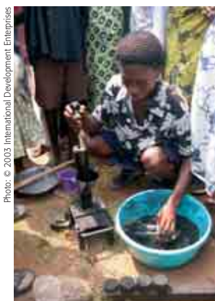
Woman in the Jukwa market in Ghana making high-density briquettes using a press designed and manufactured by MIT D-Lab.
