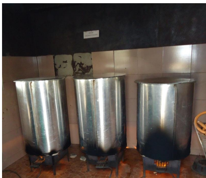
Photo 5: Picture of Improved Aluminum Boilers for Brewing Traditional Herbal Medicine Preparations
