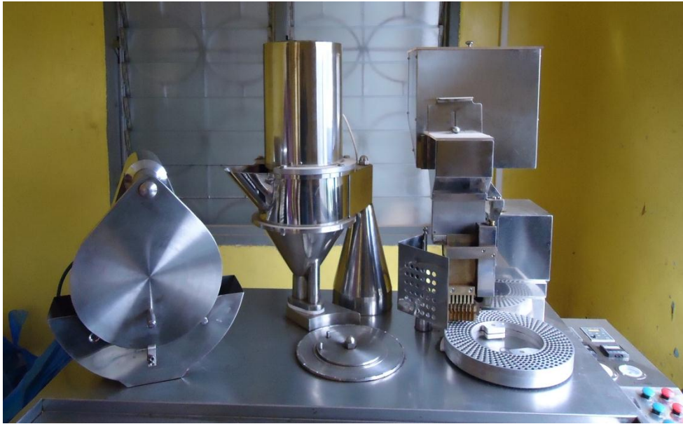
Photo 6: Picture of capsule filling machine, for the production of traditional medicine in capsules
