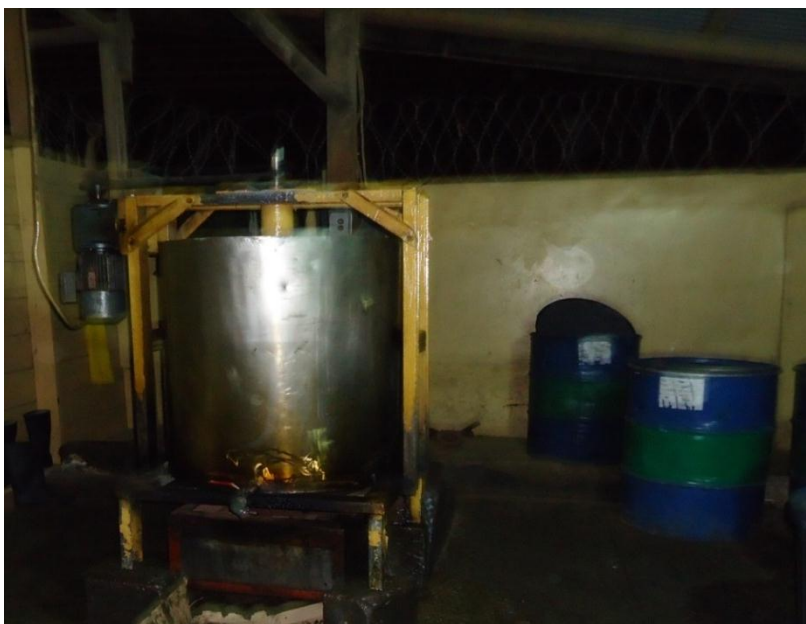
Photo 10: Picture of mixing machine for mixing herbal soap
