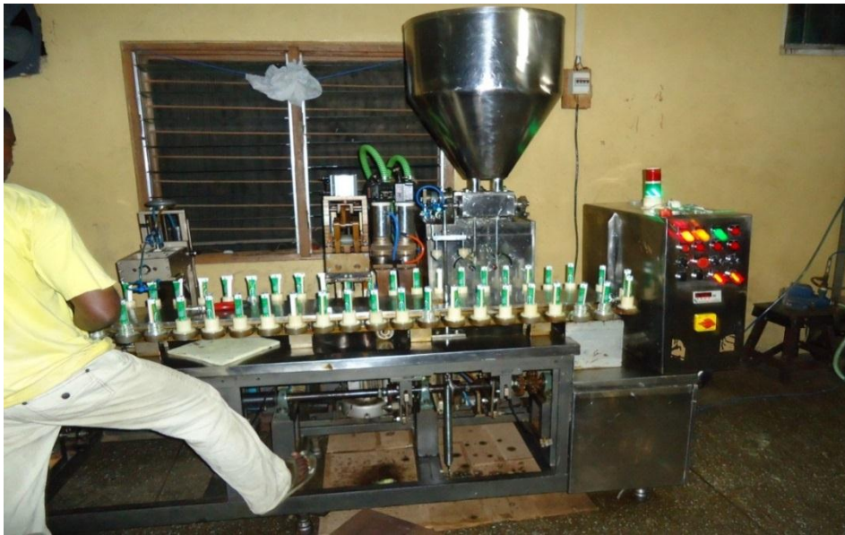
Photo 9: Picture of tube filling machine being used to fill tubes with creams
