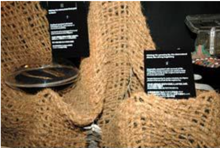
Geotextile net utilizing coconut shell fibers (Philippine Pavilion)
