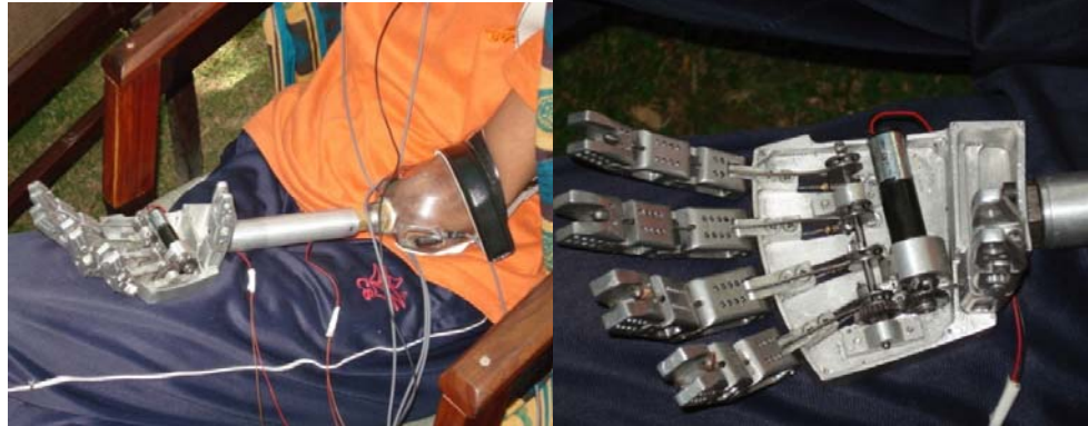
Figure 1. On the left: Testing the Prototype on the Patient. On the right: The fabricated robotic hand
