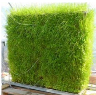
Vertical Green Biobed for the efficient degradation of pesticides From University of Geneva
