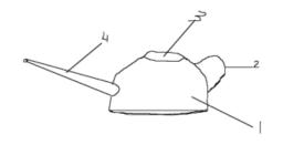
A device for watering plants having: a water-containing portion (1), a handle (2), an opening with a lid (3) and a spout (4).
